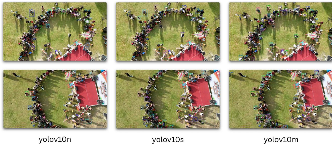
Fig 6. Example detections from YOLOv10n, YOLOv10s, and YOLOv10m models on identical drone surveillance frames. Larger models (s and m) capture more individuals with higher bounding-box coverage compared to the lightweight YOLOv10n.
