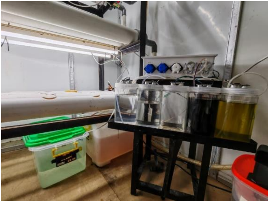
Figure 1 Physical hydroponic prototype showing channels, reservoir, solution containers, and electronics enclosure.
